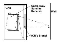
To help the VCR's signal reach your cable box or direct-to-home satellite receiver, place the VCR and your equipment near each other. You might also have to adjust the position of your cable box or direct-to-home satellite receiver as shown above.
